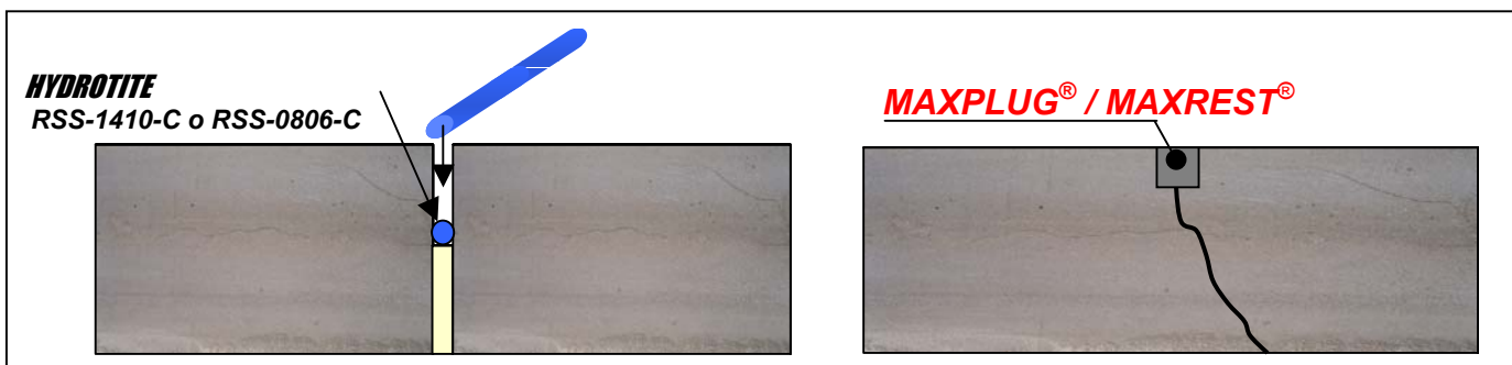
Figure 4. A) Placing of water-swelling profiles for expansive joints in cured concrete. B) Repair of cold joints in cured concrete
